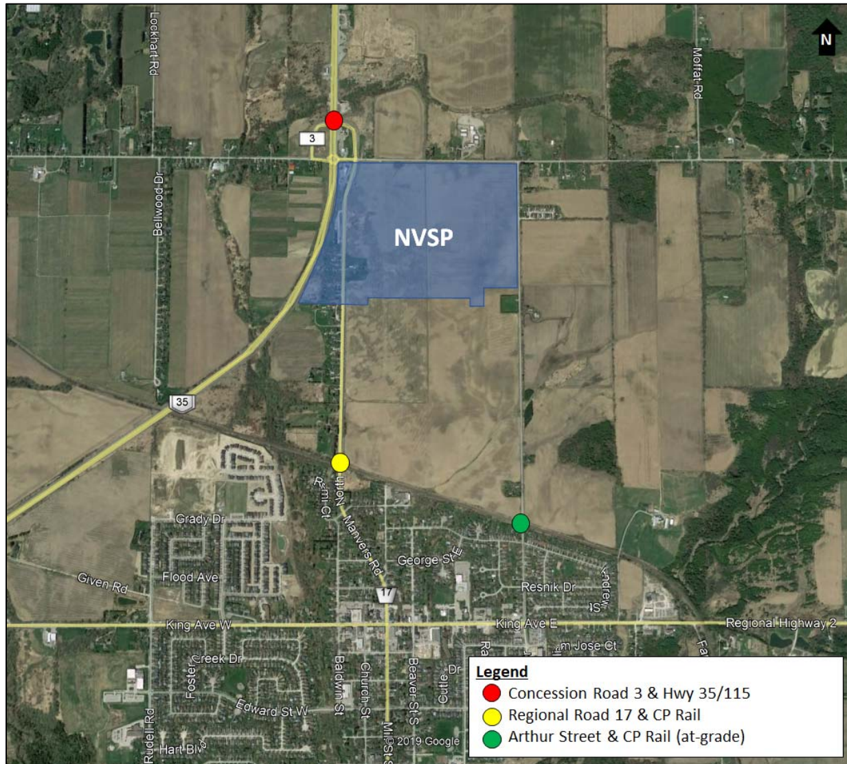
Figure 9: At-Grade and Grade-Separated Crossings within Study Area
