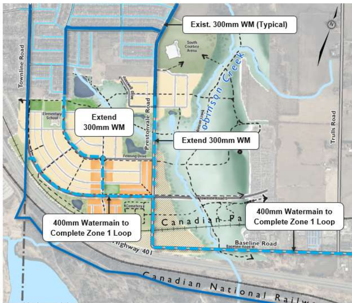
Figure 5: Planned Water Distribution Upgrades
