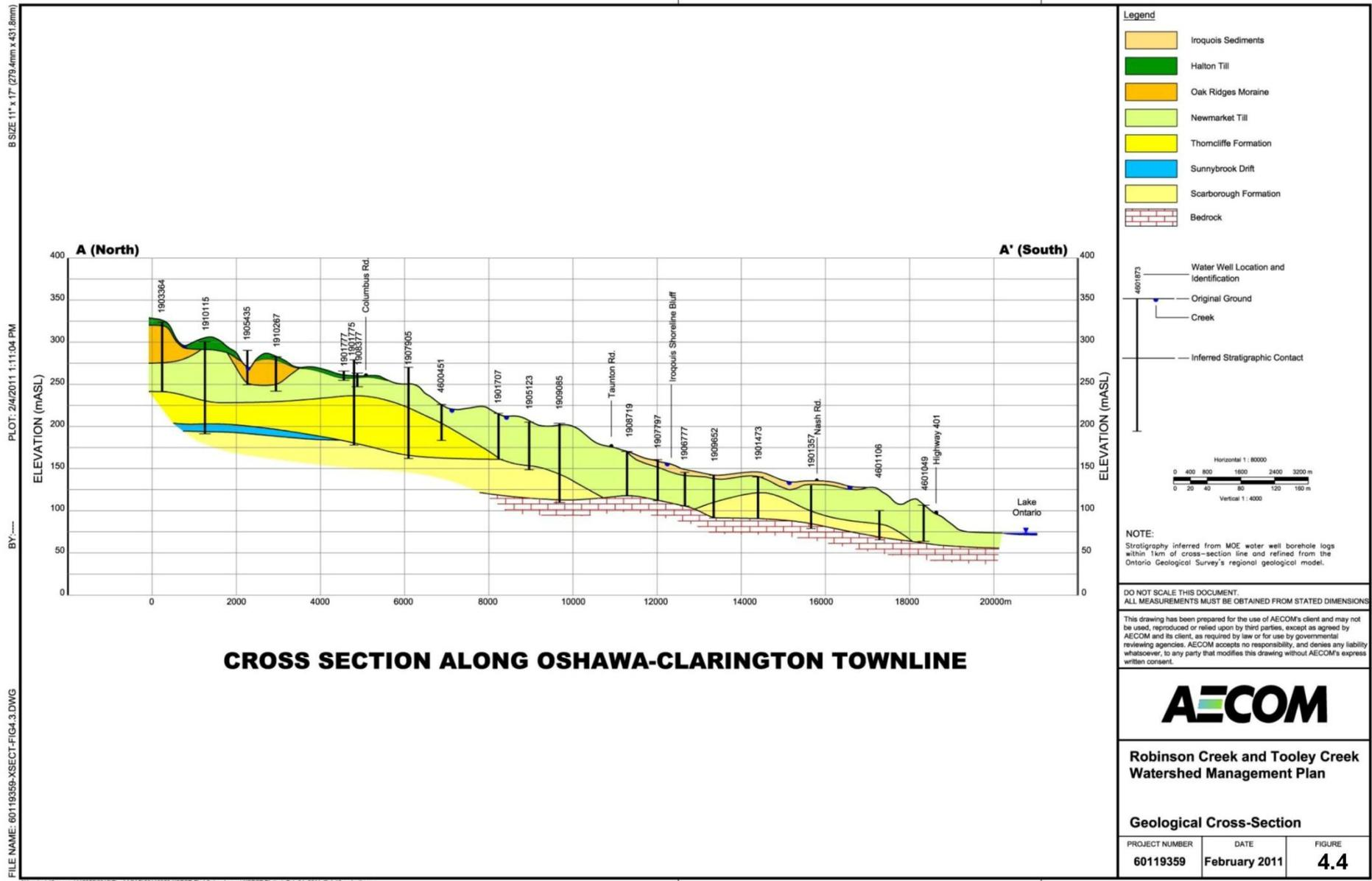
Figure 4.4 Geological Cross-Section
