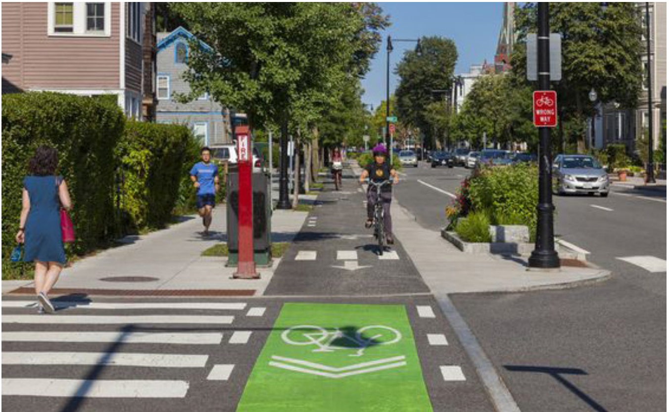
Figure 32: Example of a protected bicycle facility, separated by physical buffers to the vehicular and pedestrian portions of the right-of-way.
