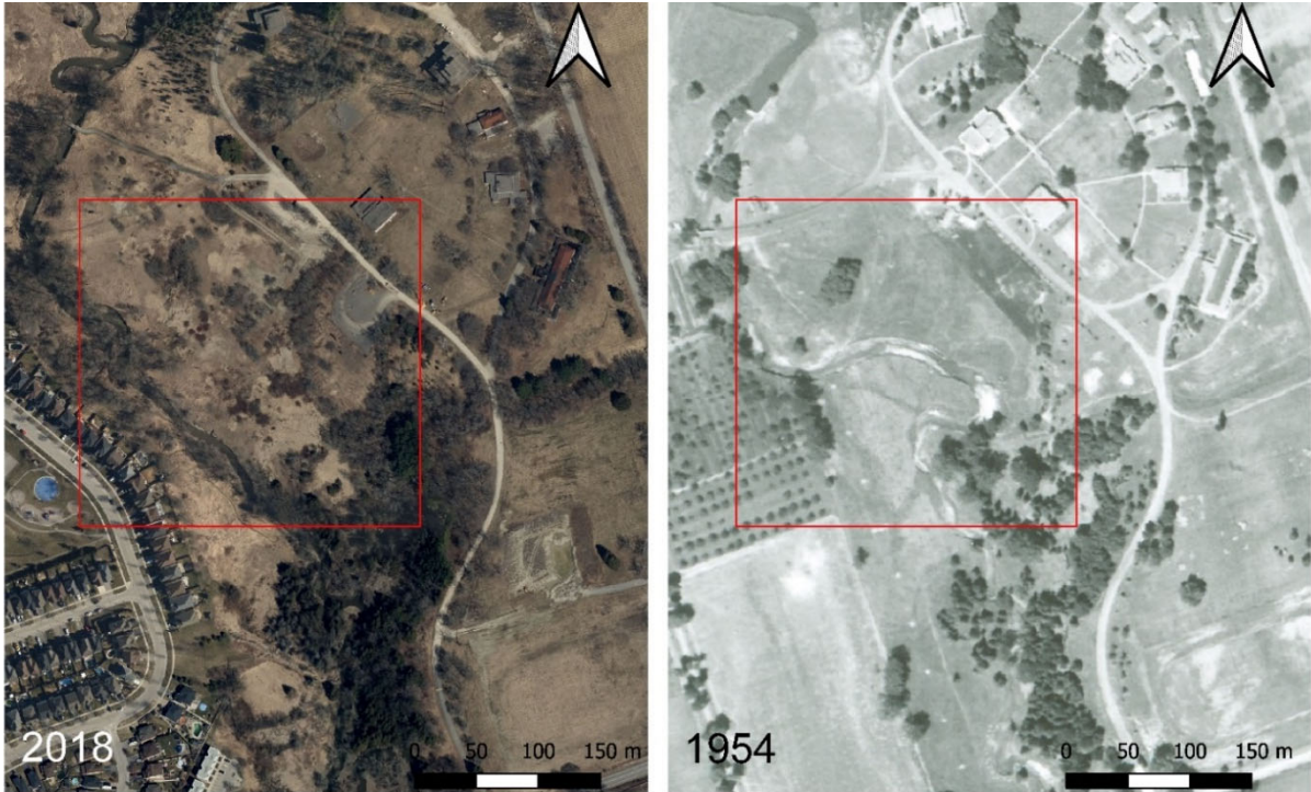
Figure 3-39: Evidence of Historic Channel Realignment Near Concession St and Lambs Rd.
