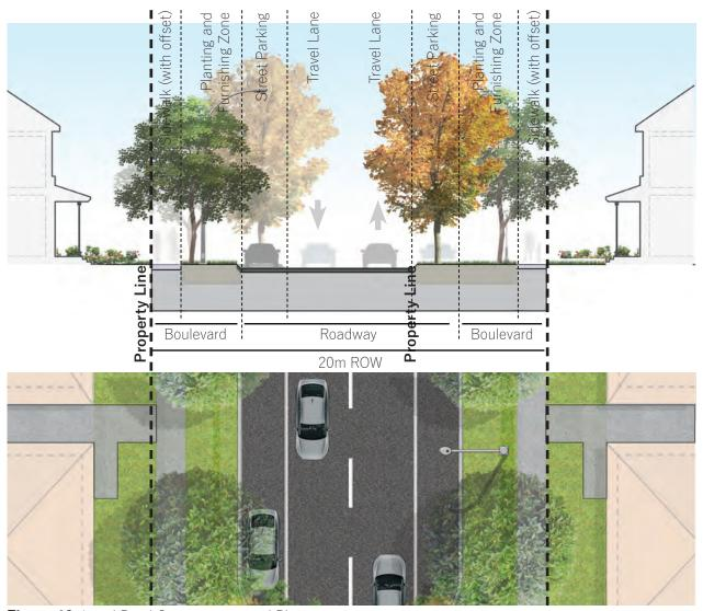
Figure 48: Local Road Cross-section and Plan
