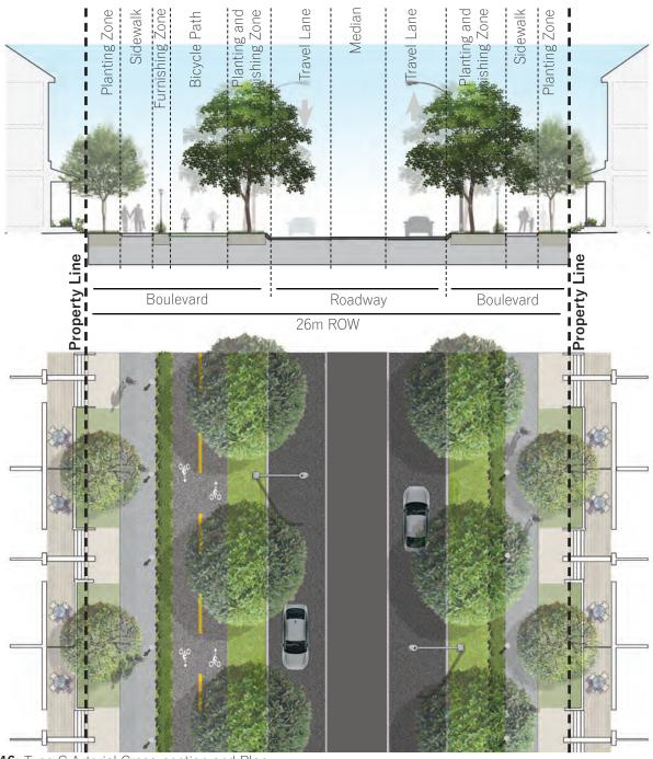
Figure 46: Type C Arterial Cross-section and Plan
