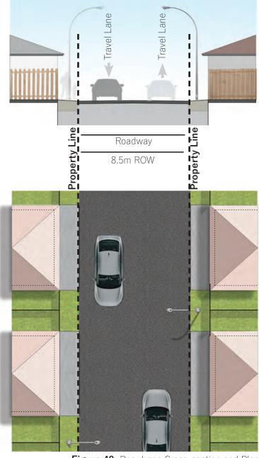
Figure 49: Rear Lane Cross-section and Plan
