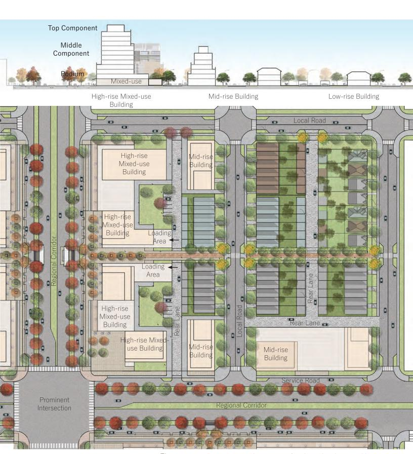
Figure 15: Height, Massing and Transition of High- and Mid-rise Buildings
