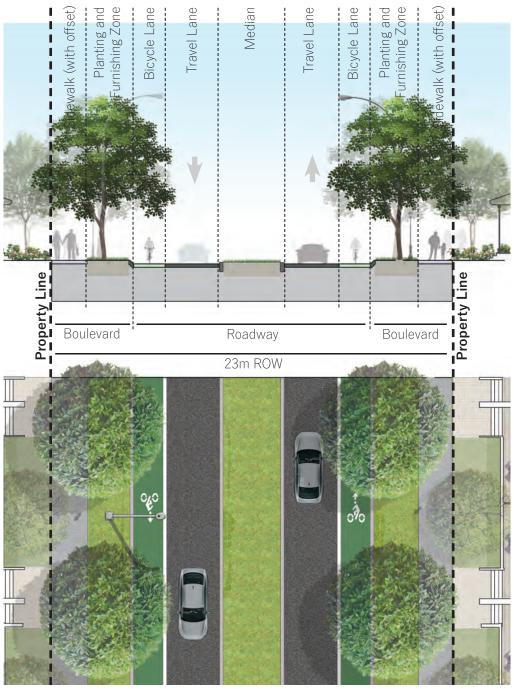
Figure 47: Collector Road Cross-section and Plan
