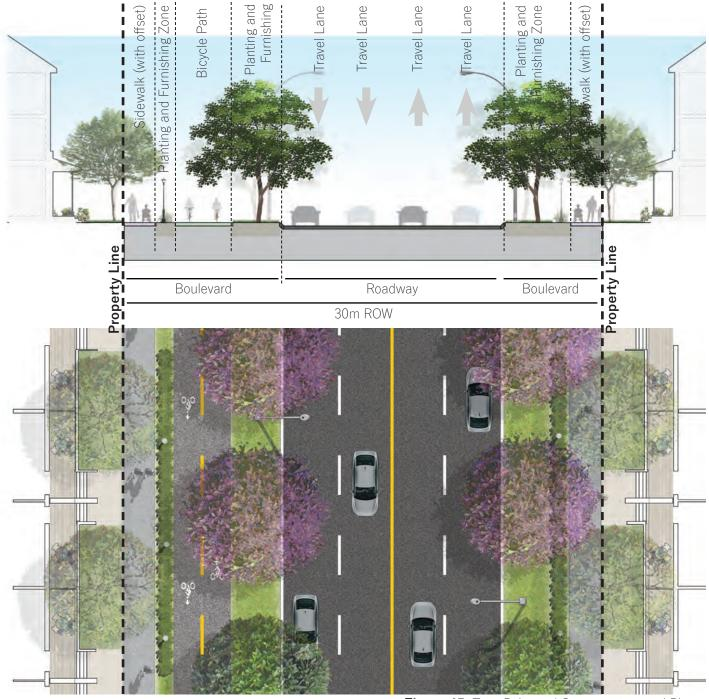
Figure 45: Type B Arterial Cross-section and Plan
