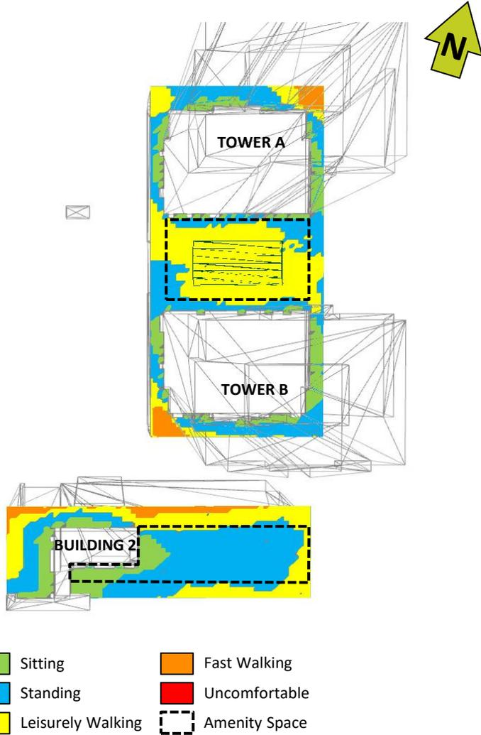
Figure A3a: Proposed Configuration – Pedestrian Wind Comfort Spring – Amenity Terraces
