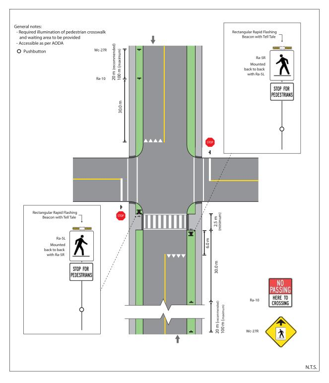
Figure 36: Pedestrian Crossover Level 2 Type C – Intersection (2-way)
