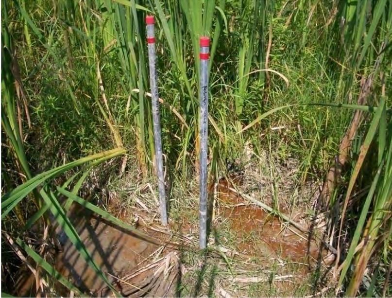
**Photo 1. Mini-piezometer Wetland Pair at RC-MP1**
