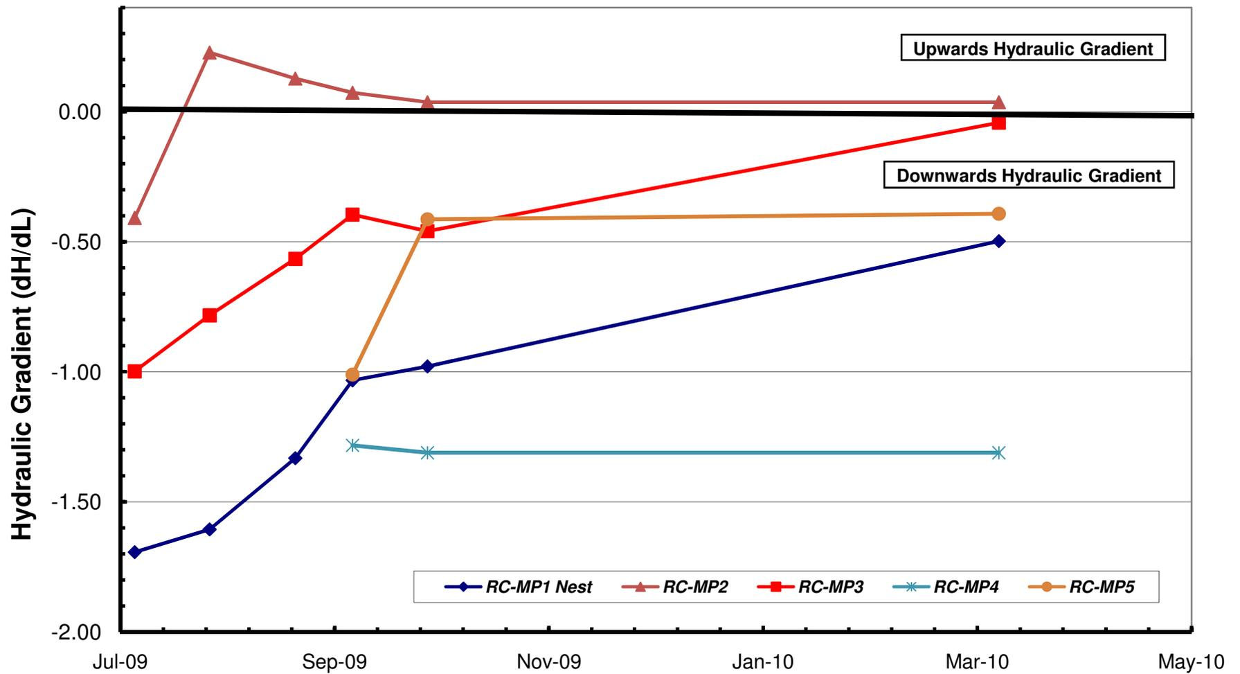
Hydraulic Gradients in Mini-Piezometers (Robinson Creek Watershed)
