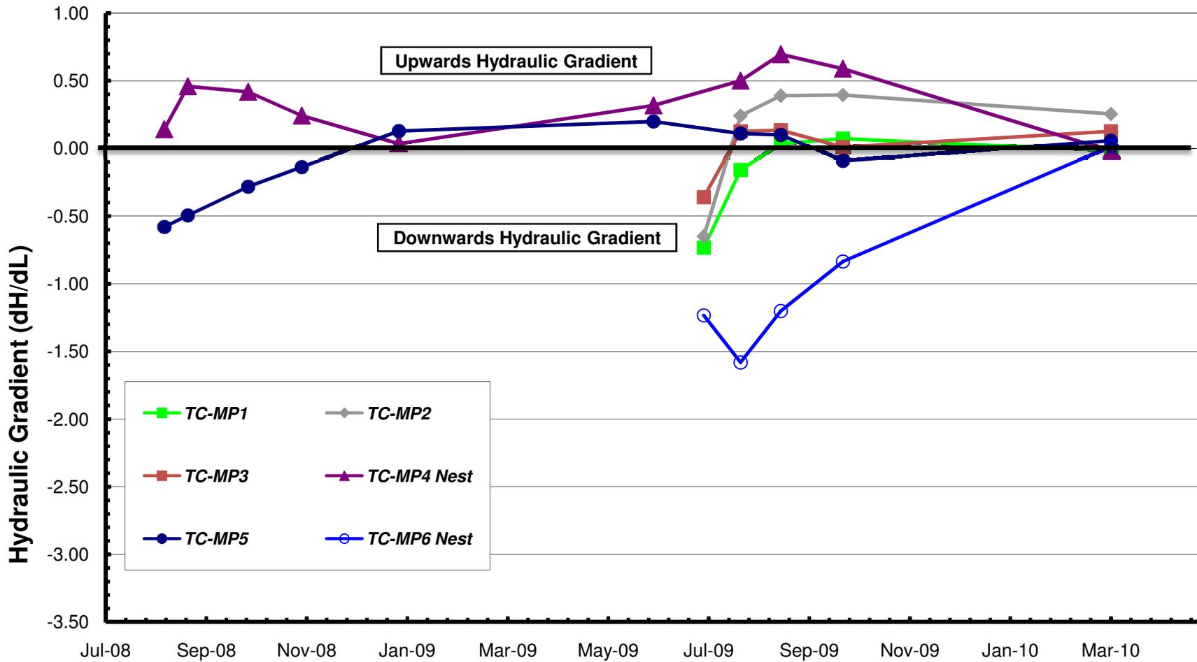
Hydraulic Gradients in Mini-Piezometers (Tooley Creek Watershed)
